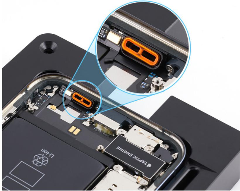
2. If the rubber gasket is out of position, use ESD-safe tweezers to reposition it.
