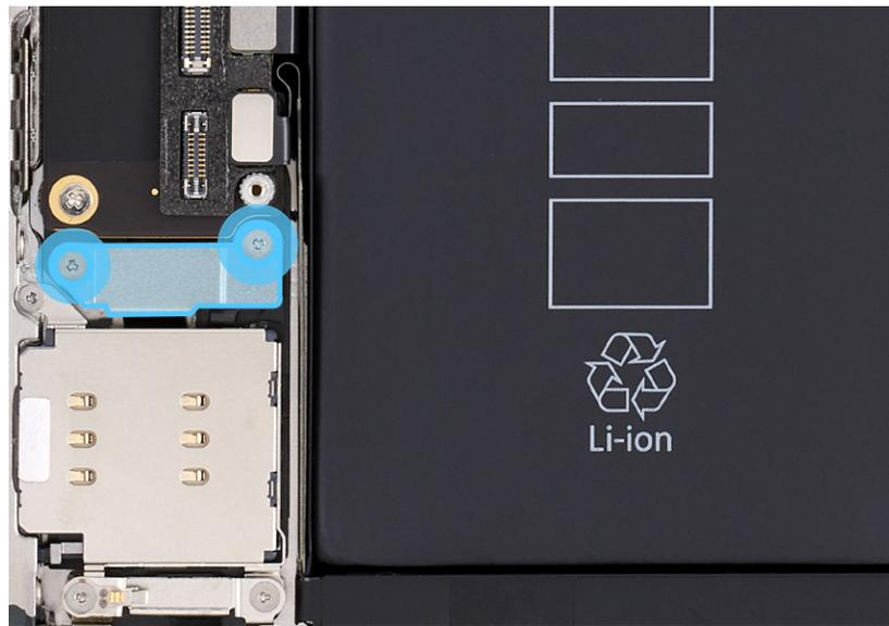
6. Use a torque driver and the Micro stix bit to remove the two trilobe screws from the Taptic Engine connector cowling. Set aside the screws.
