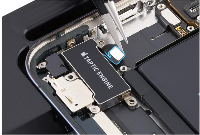
15. Use ESD-safe tweezers to remove the Taptic Engine.
