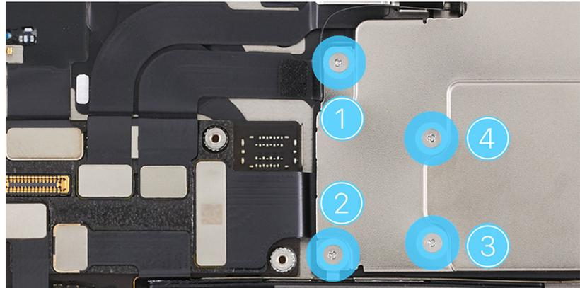
4. Use ESD-safe tweezers to remove the camera cowling. Save the cowling for reassembly.
