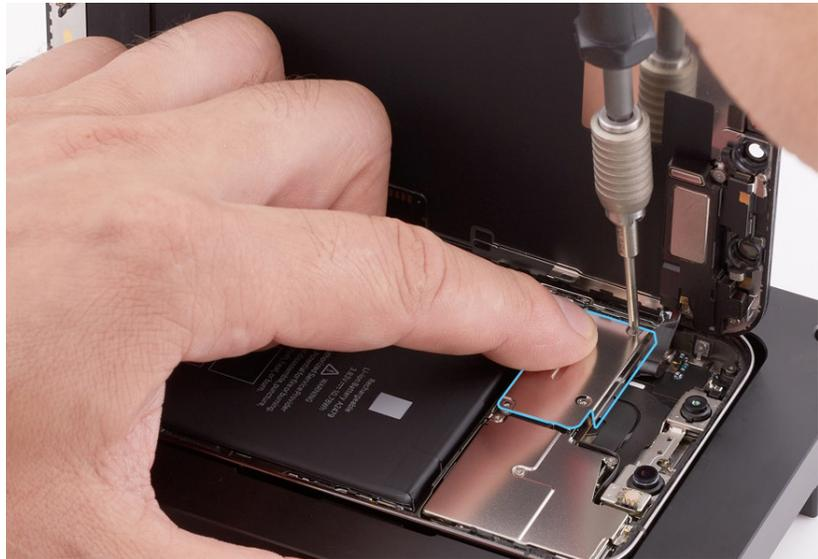
25. Use ESD-safe tweezers to remove the upper cowling. Save the cowling for reassembly.
