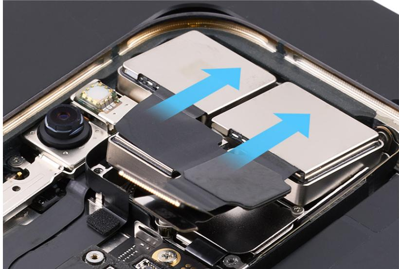
3. Press the end of the bottom camera flex cable to the connector.
