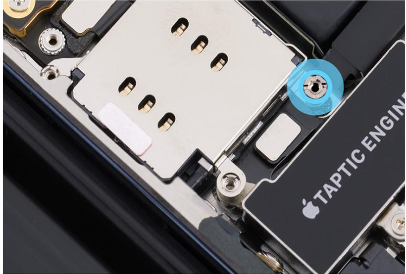
11. Tilt up the SIM reader and lift it out of the enclosure.
