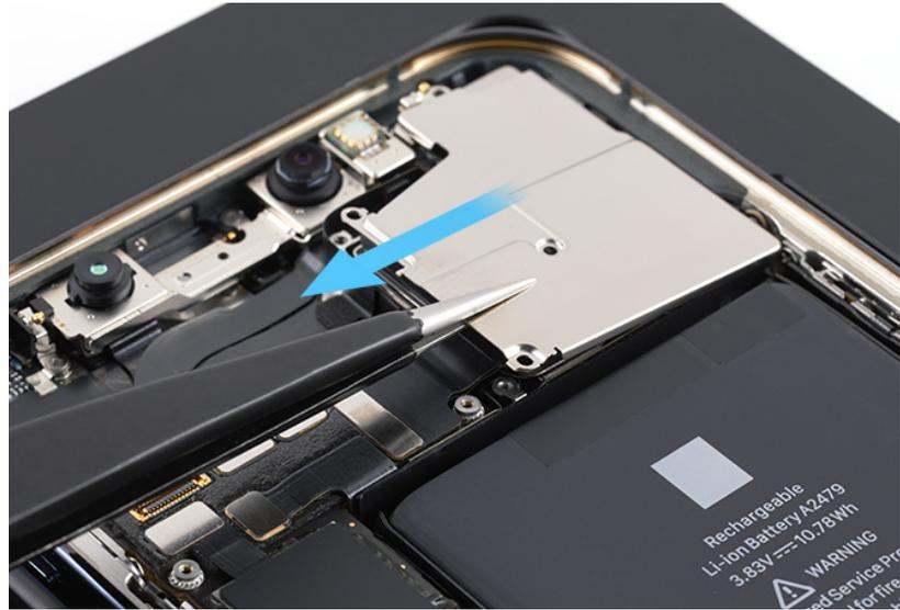
5. Use ESD-safe tweezers to gently lift the end of the top camera flex cable off the connector.
