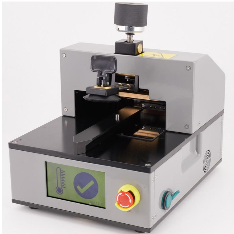
3. Gently insert the iPhone into the heated display pocket with the display faceup and the Lightning connector facing the bottom of the pocket.
