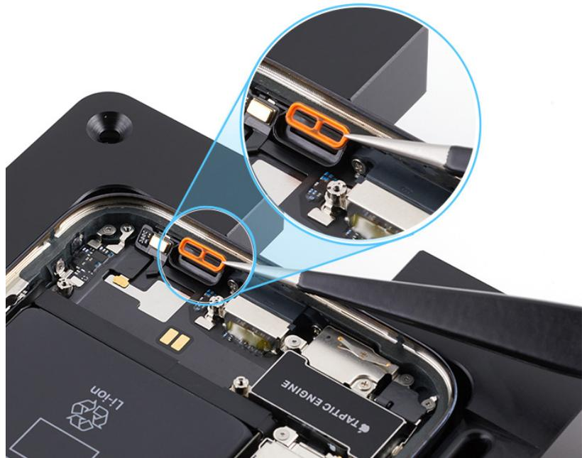
3. Rotate the repair tray. Tilt down the bottom edge of the speaker and lower it into the enclosure.
