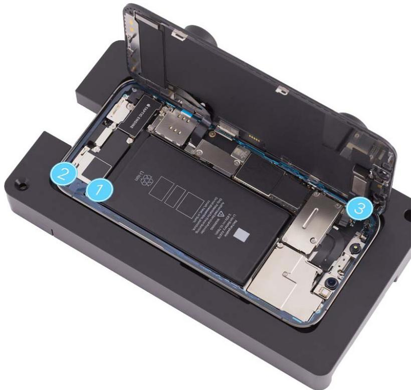
20. Inspect the display adhesive to ensure that it's in the correct position and not damaged or wrinkled. If the adhesive is damaged, remove it and apply replacement adhesive.
