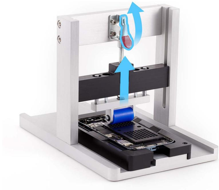
10. Position the repair tray and enclosure onto the battery press with the right slot over the pin.
