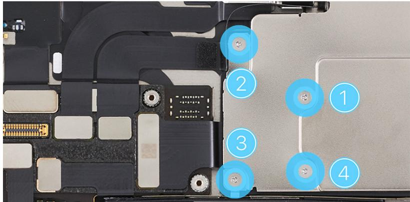
8. Use the gray torque driver and JCIS bit to install one new crosshead screw into the camera cowling.
