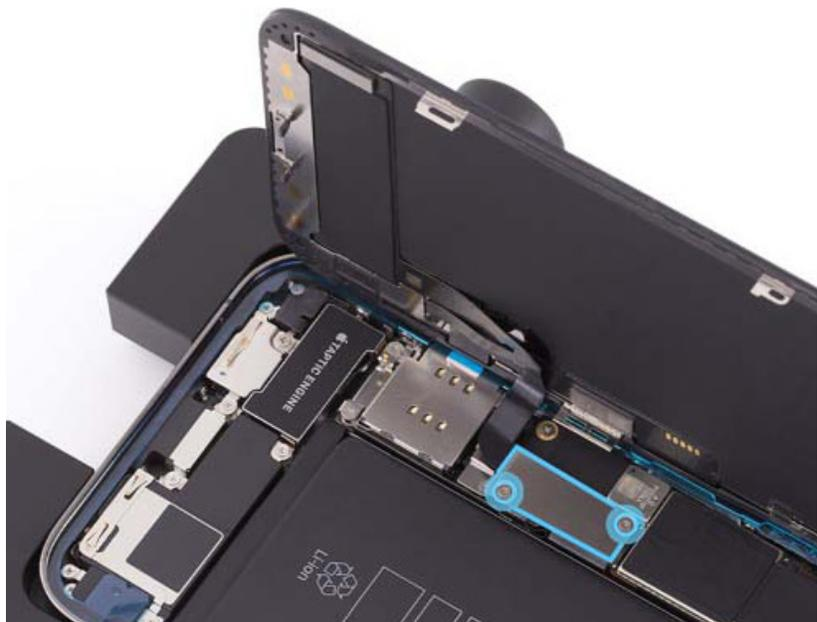
17. The upper cowling has a tab near the second screw hole (2) that fits into a slot near the camera cowling. Use ESD-safe tweezers to fit the tab into the slot. Then lower the cowling over the end of the receiver flex cable.
