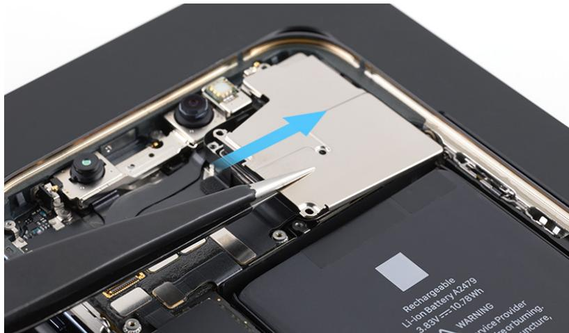
7. Use the green torque driver and Micro stix bit to install four new trilobe screws into the camera cowling in the order shown.
