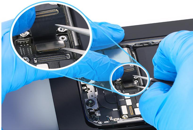
7. Gently hold the flex cables together and lift the cameras out of the enclosure.
