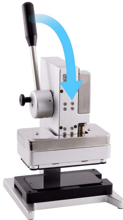
26. Wait until the timer on the display press beeps. Pull down the lever (1) and pull out the release knob (2). Then lift the lever (3).
