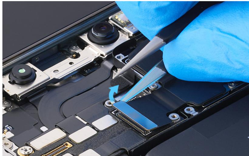
6. Use ESD-safe tweezers to gently lift the end of the bottom camera flex cable off the connector.
