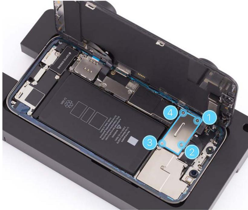
19. Peel the first strip of the middle release liner (1) counterclockwise, starting near the bottom of the enclosure. Peel the second strip (2) clockwise, starting near the bottom of the enclosure. Peel the third strip (3) counterclockwise, starting near the top of the enclosure.
