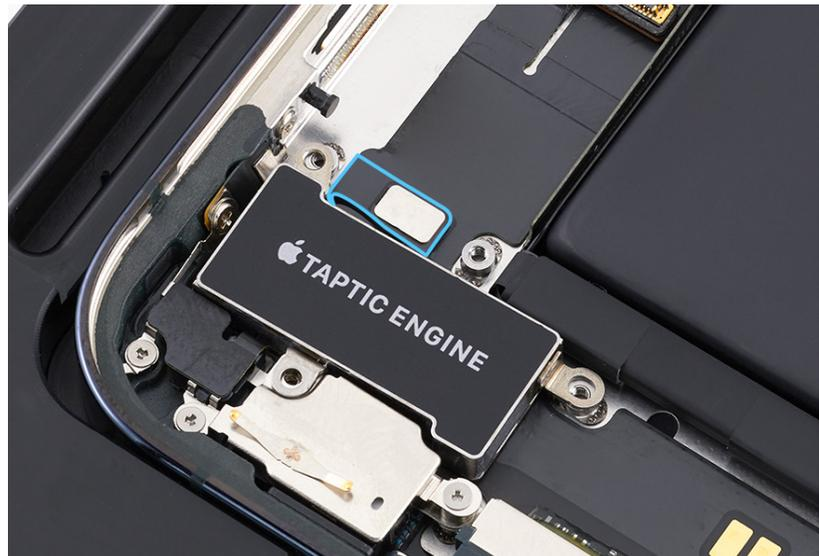
3. Use the green torque driver and JCIS bit to install one new crosshead screw into the Taptic Engine.
