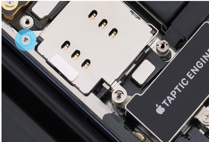
10. Use a torque driver and the super screw bit to remove the super screw from the lower right corner of the SIM reader. Set aside the screw.
