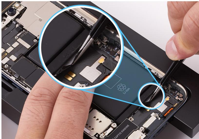
5. Keep the tweezers close and parallel to the battery and twist until you see white adhesive strip on the tweezers.
