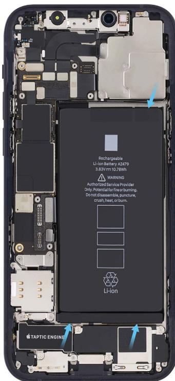
16. Slightly lift the battery with the black stick just enough to grasp underneath the battery.
