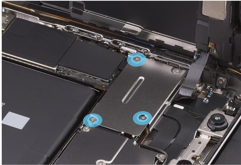
24. Hold the upper cowling in place and use a torque driver and the Micro stix bit to remove the last trilobe screw. Set aside the screw.
