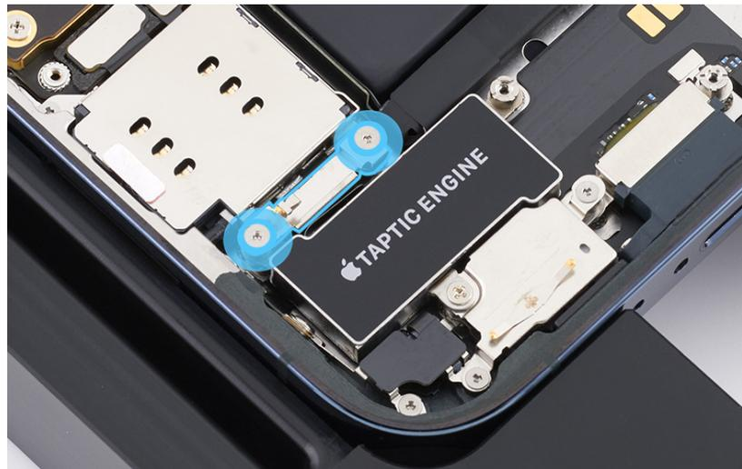
8. Use ESD-safe tweezers to lift the end of the SIM reader flex cable off the connector.
