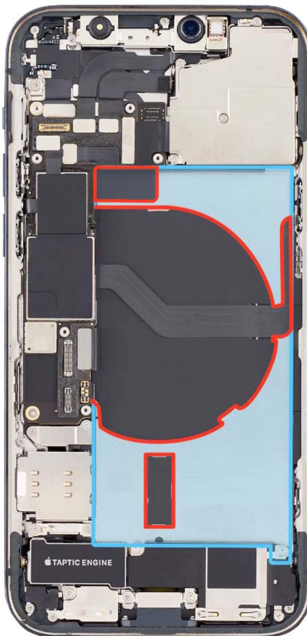
4. Peel the pink release liner from the underside of the replacement battery.
