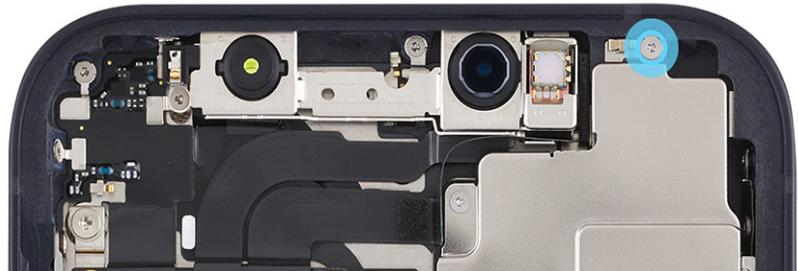
3. Use a torque driver and the Micro stix bit to remove the four trilobe screws from the camera cowl in the order shown. Set aside the screws.
